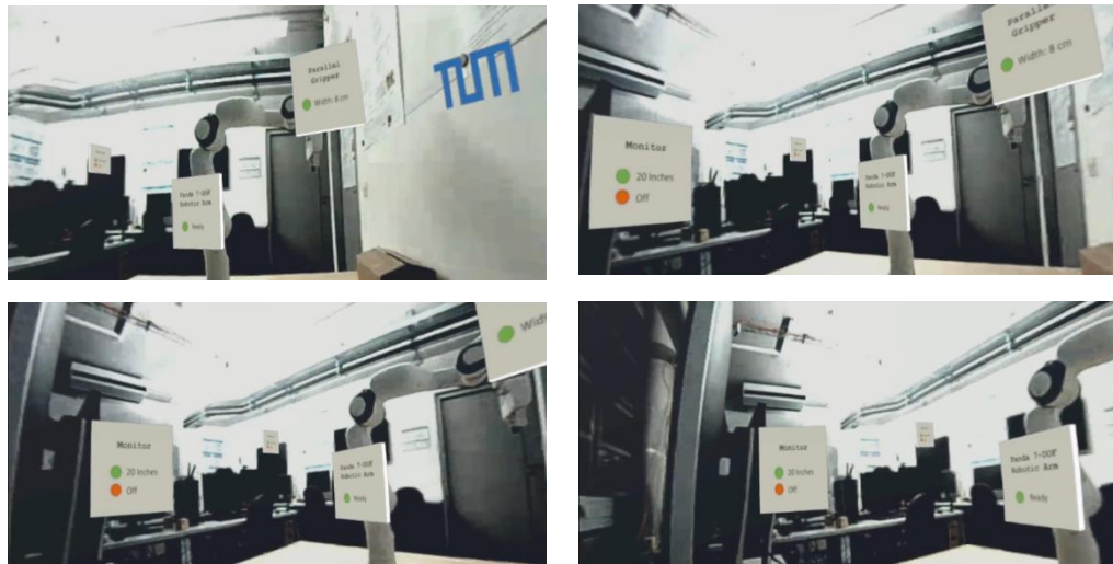
Figure 7. Corrected Hologram rendering after applying fisheye distortion
