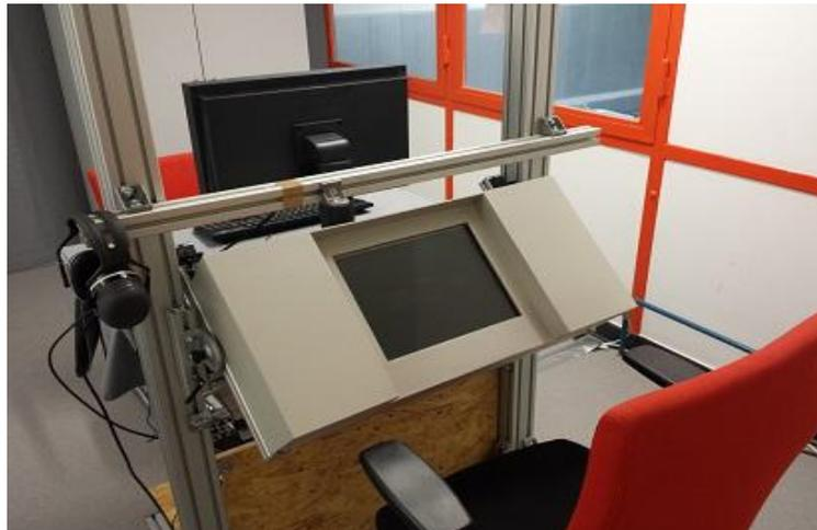
Figure 1. Stationary touch screen mock-up used in this experiment
