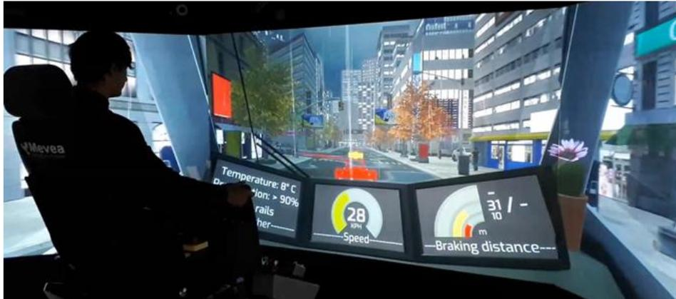
Figure 2. A virtual reality based SmartTram simulator. Tram operator's view in an autumn-evening lighting condition in an urban city environment. The rain and fallen leaves on the tramlines affect acceleration and stopping distance of the tram
