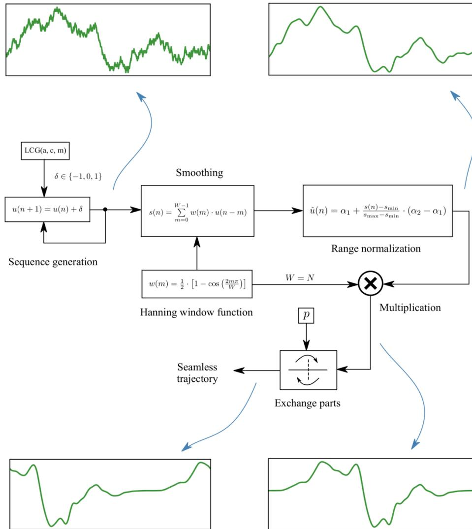
Figure 4. Diagram of the proposed scheme
