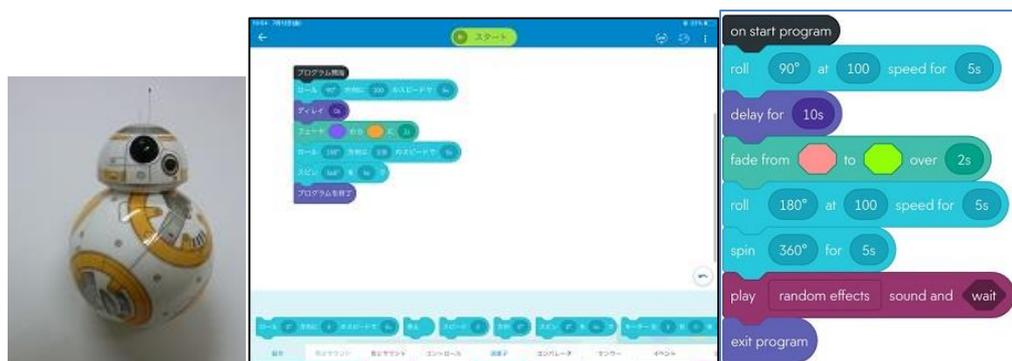
Figure 2. BB-8(left), interface of SpheroEdu for coding with blocks (center) and sample code (right)
