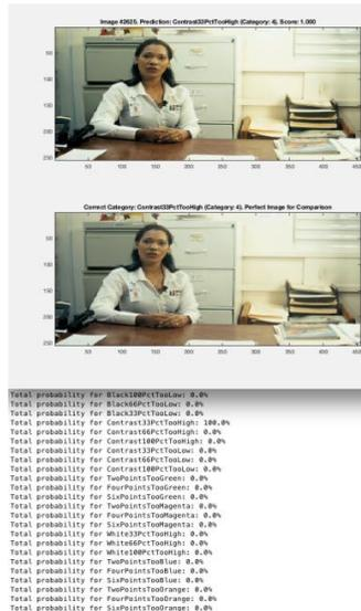
Figure 5. Correct classification that the source image's contrast is 33% too high. Note that the confidence in the result is 100%
