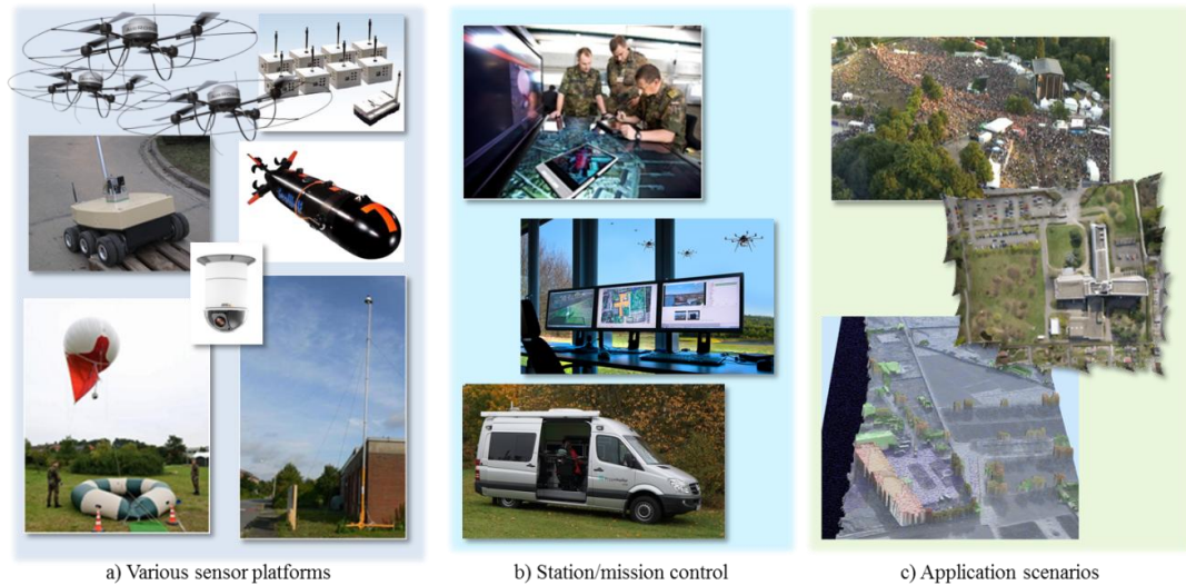
Figure 2. Example components of the interconnected system network ExBA. a) Left: various sensor platforms like quadcopters, land robots as well as stationary and mobile cameras. b) Center: various control stations. c) Right: multiple application scenarios, like supervision of public festivals, image mosaicing and change detection for property surveillance or automatic 3D terrain generation
