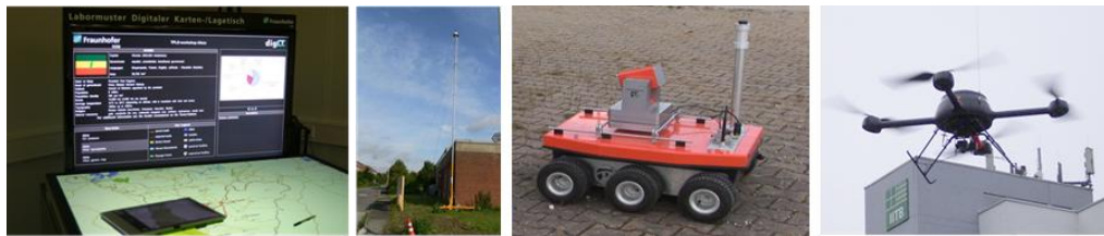
Figure 1. Some components of the experimental system for image exploitation ExBA, (from left to right) digital situation desk, stationary dome camera, land robot, quadcopter drone
