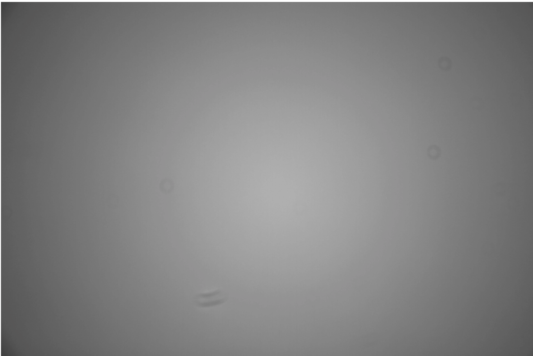
Figure 4. A typical flat field exposure can be taken from the bright sky in daylight or from a flat illuminated wall. With the large focal length of a telescope, it is assumed, that the intensity of the bright sky will not vary within the small angle of view at zenith. The effect of vignetting introduces a certain drop of intensities to the borders of the image. A few „donuts“ are also found in the image and caused by dust. The small particles may be found left in the optics or at the glass plate in front of the imaging sensor. The flat field also represents the local variation of pixel sensitivity. In a first order approximation the variations of sensitivity are compensated from a division by the flatfield exposure (which should be an averaged flatfield, if statistical image processing is applied).
