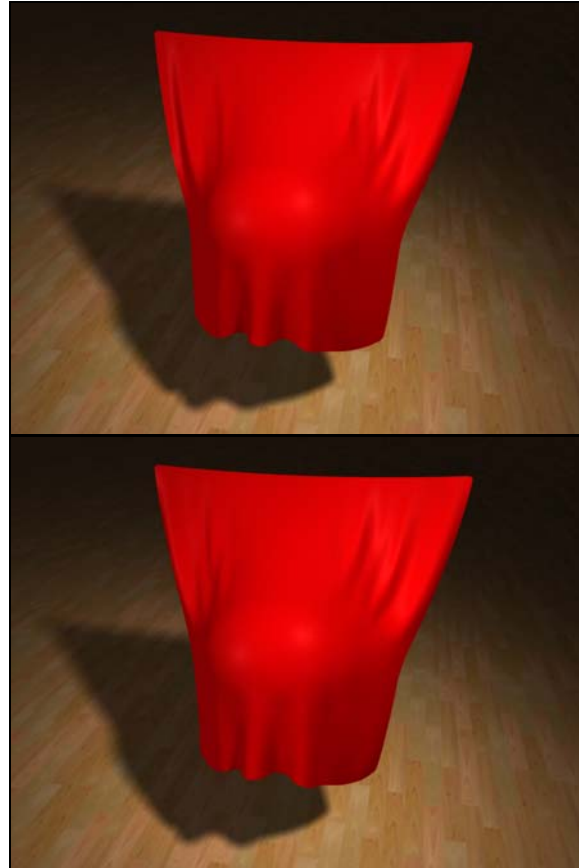
Figure 4. Simulation of a cloth model with different tolerance values in order to get a maximum allowed strain between 0.01% and 10%
