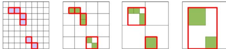
Figure 6. Mipmap construction: On the finest level, the screen-space bounding boxes (red) are set to the pixel border of each collision ray (blue), or the texels are empty otherwise. For 2 \times 2 texels the union of their boxes (green) is calculated to obtain a bounding box (red) at the next coarser level.
