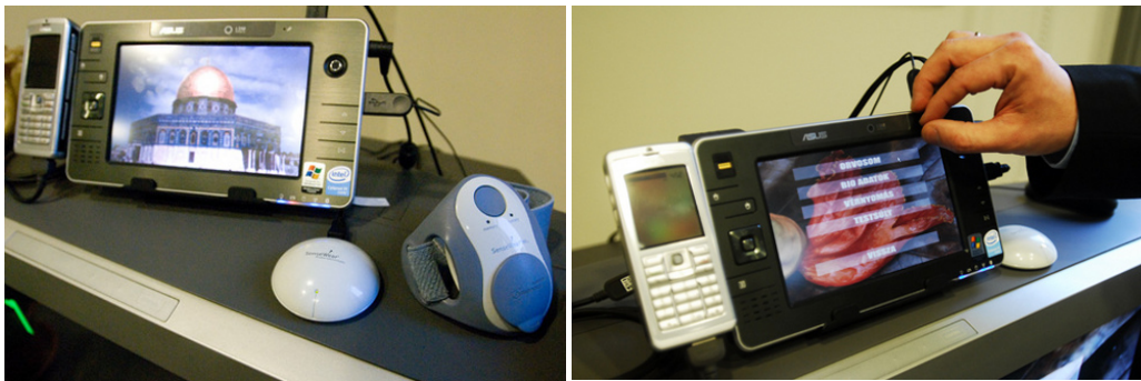
Figure 5. The central module of our AAL system on top of a television set showing family photos when not in use (left), and becoming active when touched (right)
