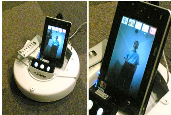
Figure 15. Home robotic platform with built in face finder, autonomous navigation, RFID and Ambient Facial Interfaces to help the elderly.
