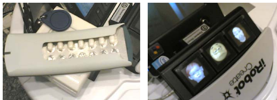
Figure 16. RFID reader with an intelligent pill dispenser placed on top of it (left); Ambient Facial Interfaces (AFIs) used to display compliance levels for medicine intake, dehydration and dietary intake, respectively (right)
